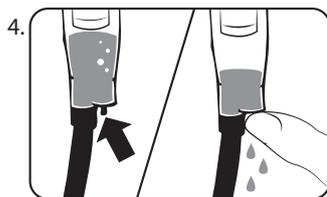
When condensation forms in the Silver Bullet™, push on the Silver Bullet™ Drain Valve to release built-up moisture. Perform this operation as often as needed – with greater frequency the higher the humidity.
